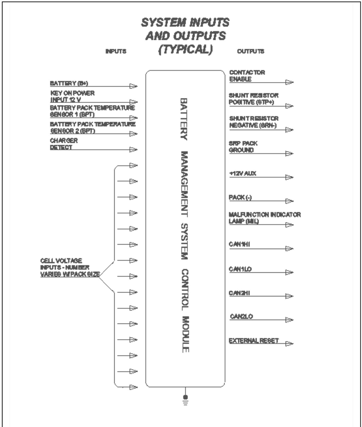
Figure 2-5 - BMS Inputs and Outputs (Typical)
