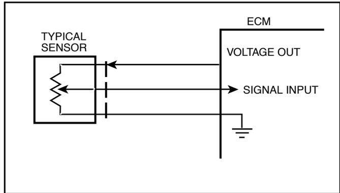
Figure 2-1 - Three-Wire Sensors
