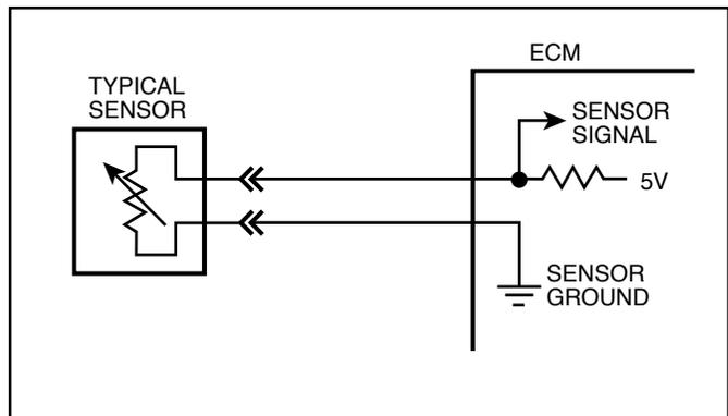
Figure 2-2 - Two-Wire Sensors
