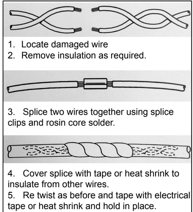
Figure 1-4 Wire Splicing Procedure
