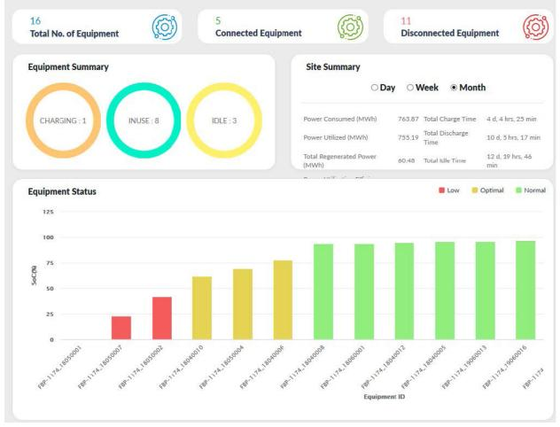
Example of dashboard that provides real time data including charge time, equipment SoC, equipment utilization, Wi Fi connection status, and more.
